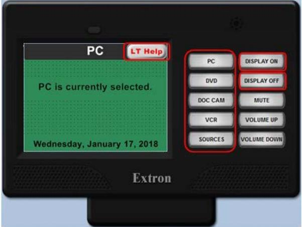
To turn the projector **ON**, press **DISPLAY ON**
