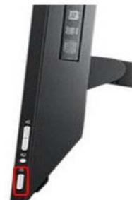
Press the power button to turn computer on
